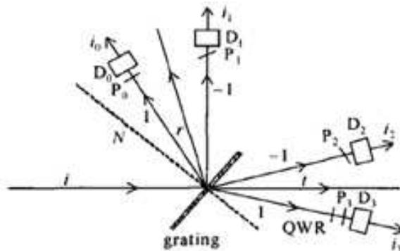
Fig. 1. The working principle of the DOAP
